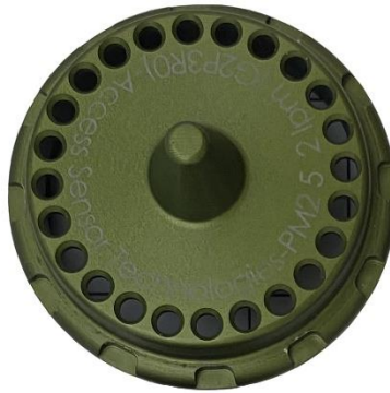
(b) Size-selective inlet PM 2.5 @ 2 L min -1 (GEN2)
