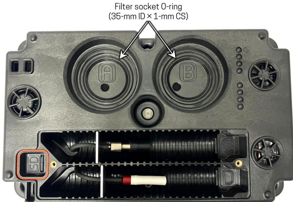
Figure 3. A photograph of the Home Health Box with the size-selective inlets, filter cartridges, sorbent media, and sorbent inlet blocks removed to show the Channel A, B, C, and D labels.
