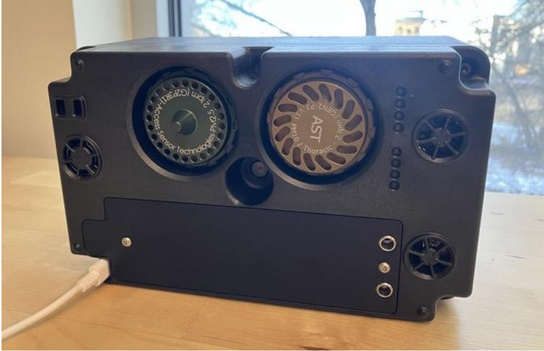
Figure 5. The Home Health Box is designed to be set down on a flat surface, as shown here, with the front of the box (i.e., the face with the inlets) facing the room during sampling (i.e., not facing towards a wall or up against any other vertical surface).
