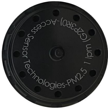
(a) Size-selective inlet PM 2.5 @ 1 L min -1 (GEN2)
