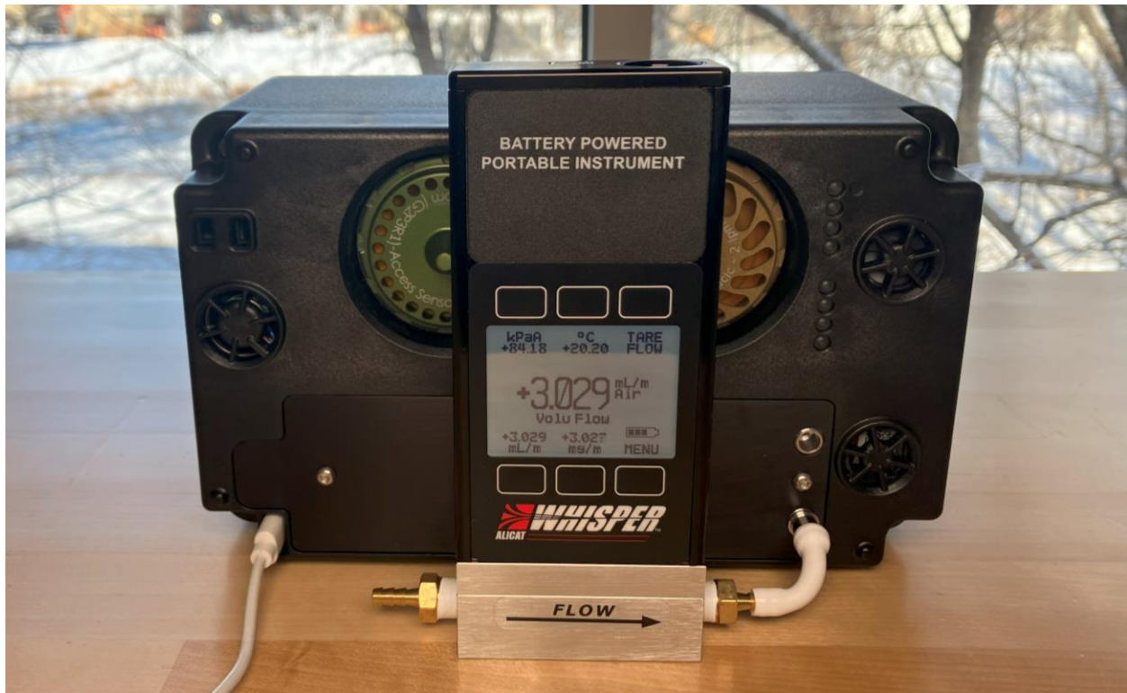
Figure 16. A photograph illustrating how to insert the sorbent inlet block calibration adapter into the sorbent inlet block and connect the adapter to a meter to check the volumetric flow rate of a sorbent sample.
