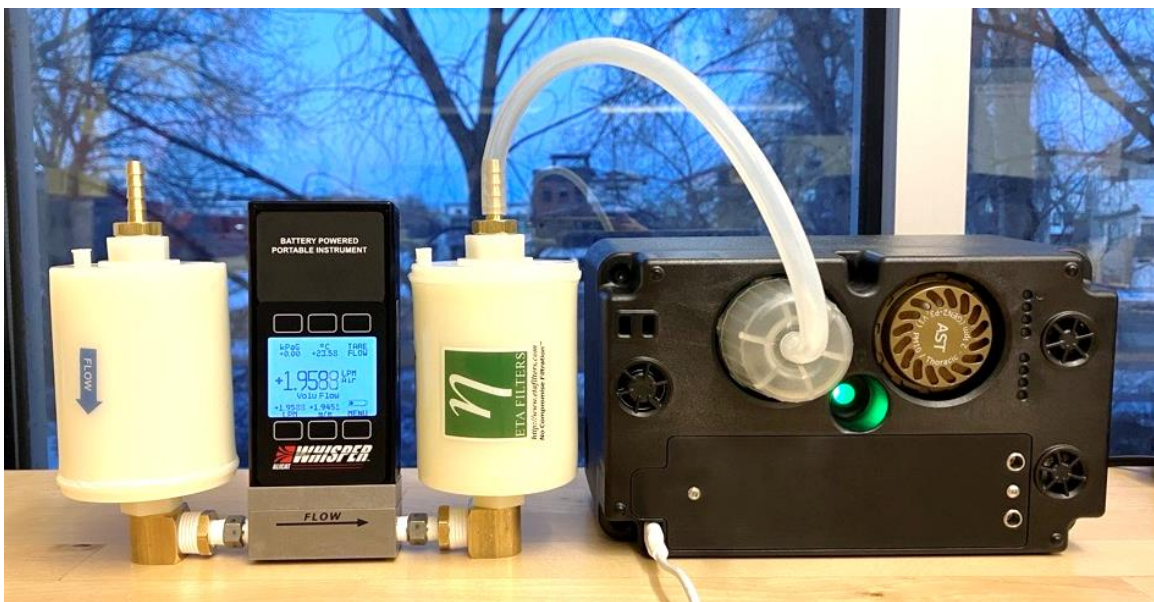
Figure 15. A photograph illustrating how to seal the filter calibration and flow adapter over a size-selective inlet and connect the adapter to a meter to check the volumetric flow rate of the filter sample.
