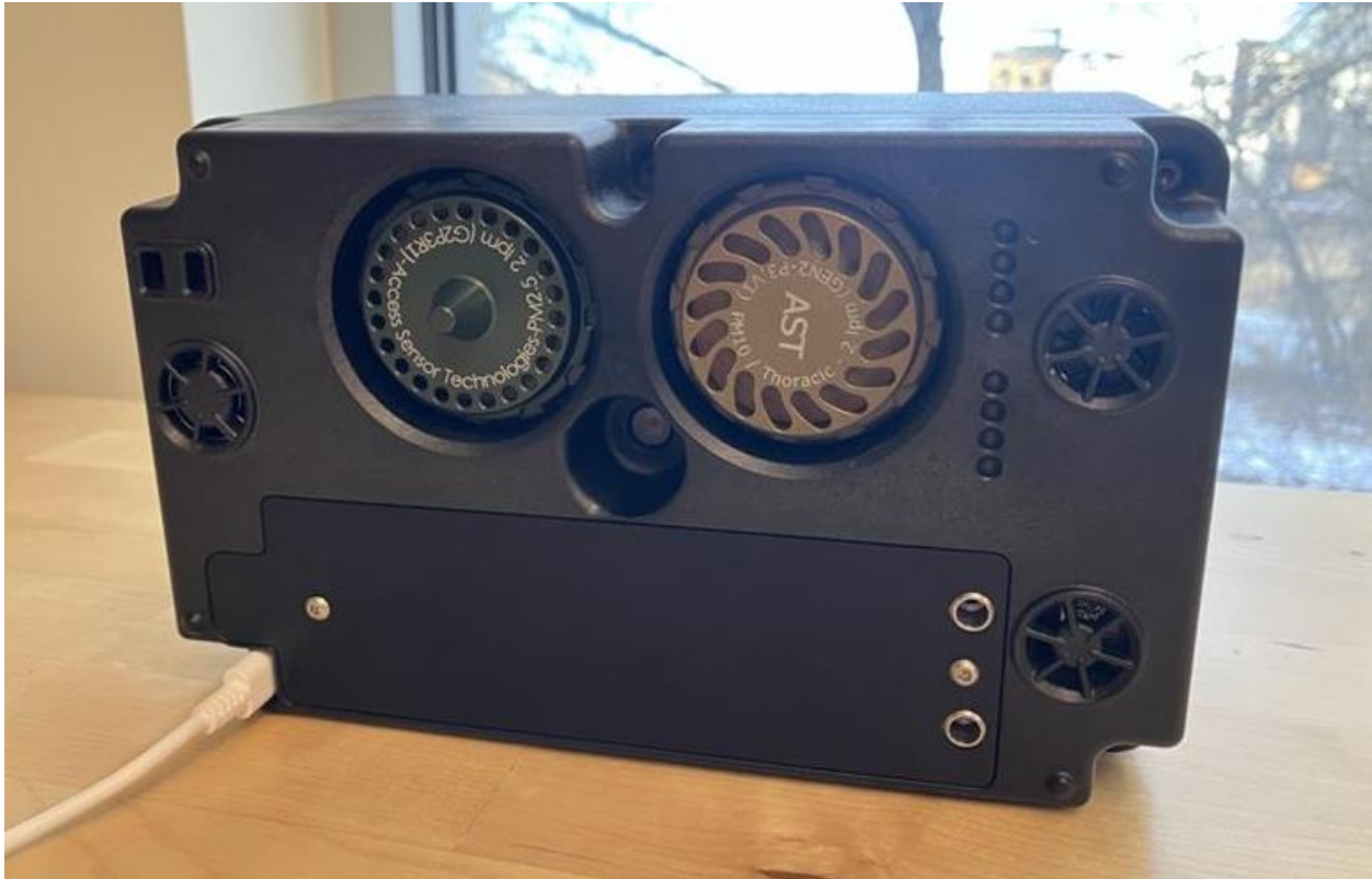
Figure 12. The Home Health Box is designed to be set down on a flat surface, as shown here, with the inlets facing the room (i.e., not facing towards a wall or up against any other vertical surface), during sampling.
