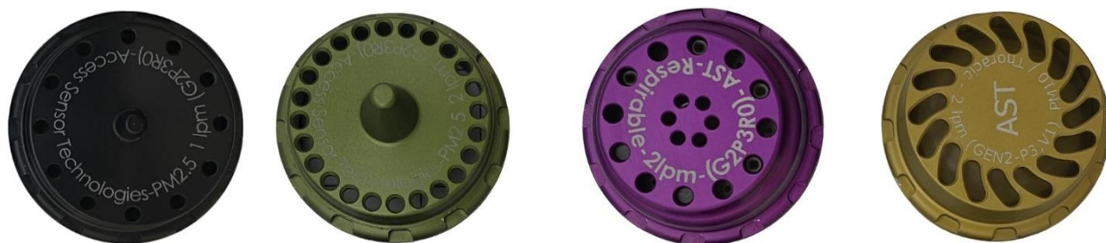
(a) PM 2.5 @ 1 L min -1 (b) PM 2.5 @ 2 L min -1 (c) Respirable PM @ 2 L min -1 (d) PM 10 @ 2 L min -1
