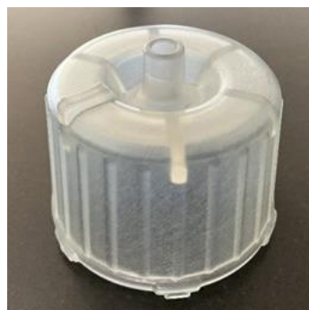
Figure 6. Filter inlet flow check adapter.
