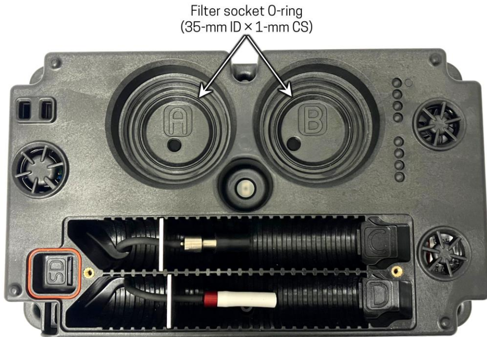
Figure 3. An HHB with the size-selective inlets, filter cartridges, sorbent media, and sorbent inlet blocks removed to show the Channel A, B, C, and D labels.
