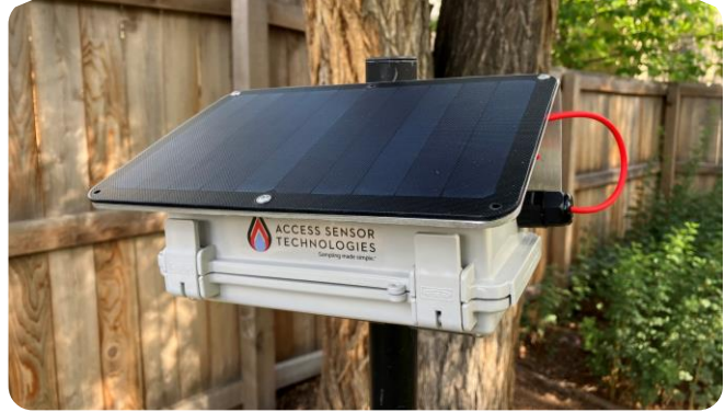
Figure 19. Left: View of the UPAS outdoor enclosure from the ground with a UPAS v2.1 PLUS installed. Right: A top view of the enclosure with a solar panel installed.
