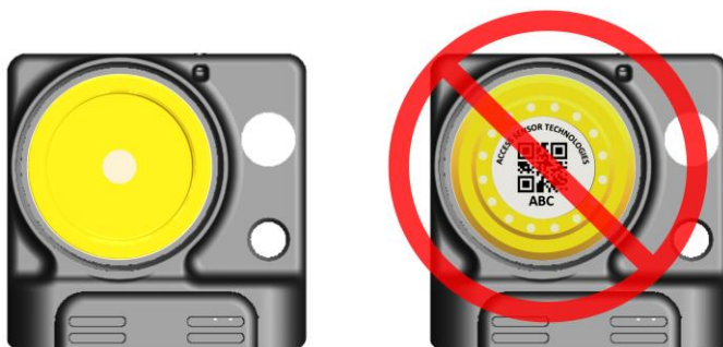
Figure 11. A filter cartridge placed in the UPAS inlet socket. The side with a ring of many small holes plus the QR code must face down. A GEN2 37-mm cartridge is shown here; installation of the 25-mm cartridge is similar.
