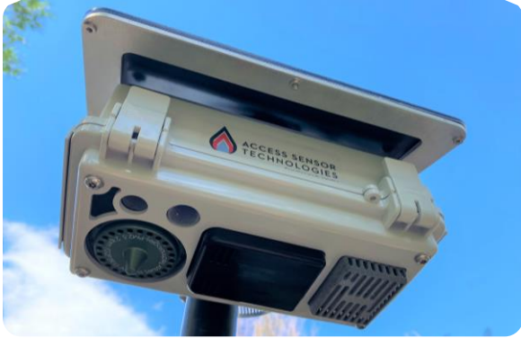
Figure 17. Left: View of the UPAS outdoor enclosure from the ground with a UPAS v2.1 PLUS installed. Right: A top view of the enclosure with a solar panel installed.
