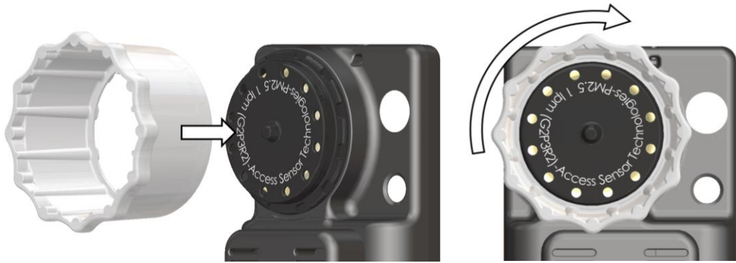
Figure 13. Attach the GEN2 Filter Inlet Tool to the size-selective inlet and turn clockwise to tighten fully.
