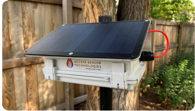
Figure 17. Left: View of the UPAS outdoor enclosure from the ground with a UPAS v2.1 PLUS installed. Right: A top view of the enclosure with a solar panel installed.
