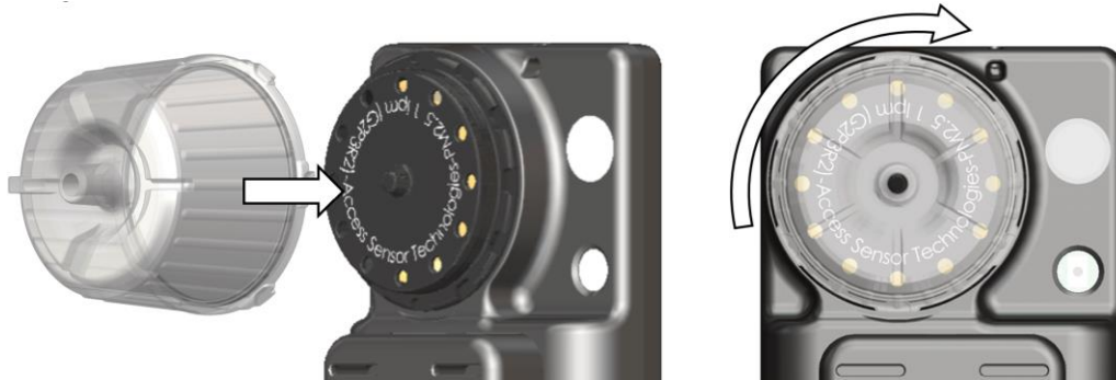
Figure 14. Attach the GEN2 Flow Check Adapter to the size-selective inlet and turn clockwise to tighten fully.
