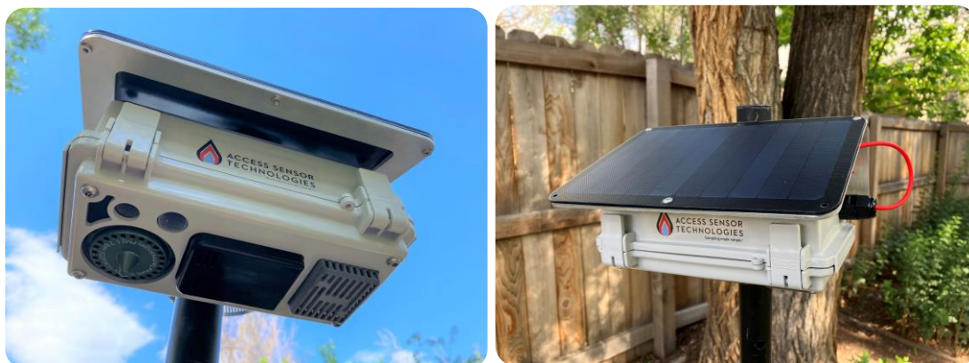
Figure 17. Left: View of the UPAS outdoor enclosure from the ground with a UPAS v2.1 PLUS installed. Right: A top view of the enclosure with a solar panel installed.
