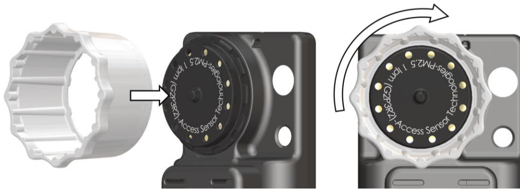
Figure 13. Attach the GEN2 Filter Inlet Tool to the size-selective inlet and turn clockwise to tighten fully.
