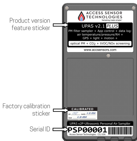
Figure 5. Back of the UPAS housing with key components identified.
