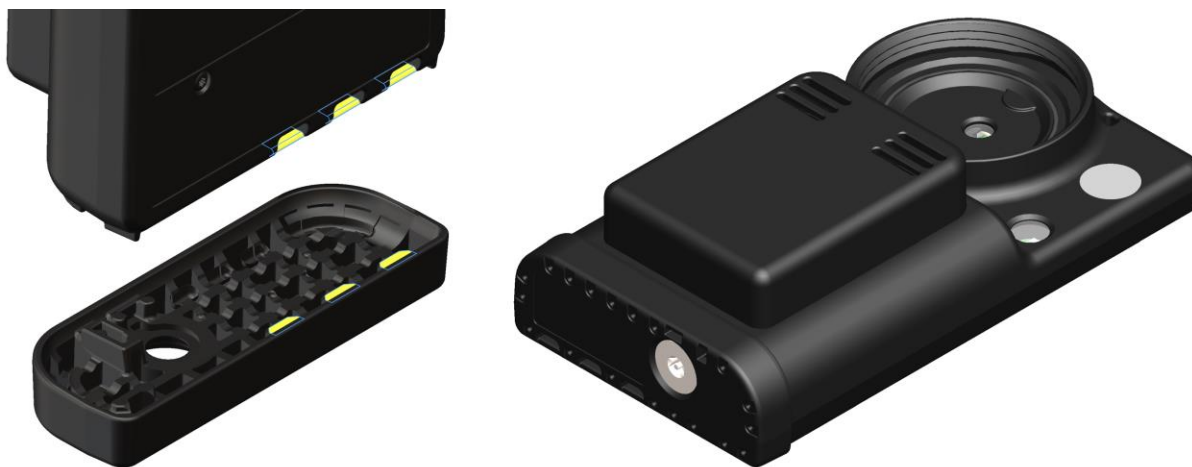
Figure 18. To install a protector on the bottom of the UPAS, hook the three tabs in the protector (highlighted in yellow on the left) into the three matching recesses in the back of the UPAS housing; then, press the protector flat against the bottom of the UPAS and secure it with a \frac{1}{4} "-20 screw (as shown on the right). Protector A is shown here as an example, but the installation procedure is the same for Protector B.
