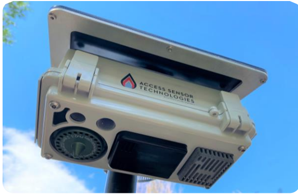
Figure 19. Left: View of the UPAS outdoor enclosure from the ground with a UPAS v2.1 PLUS installed. Right: A top view of the enclosure with a solar panel installed.
