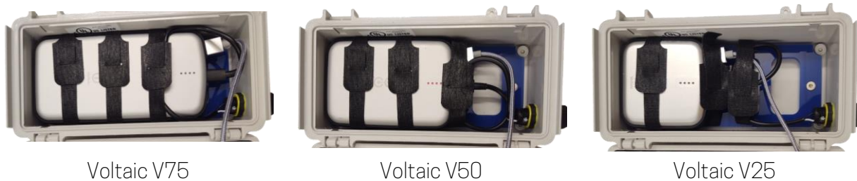
Figure 9. Voltaic Systems V75, V50, and V25 battery packs installed in the Outdoor Enclosure. These batteries are shown with the black USB-C cable connected to the USB-C charge input port on the top end of the battery (to charge the external battery pack) and a silver USB-A to micro-USB cable connected to the USB-A charge output port on the battery.
