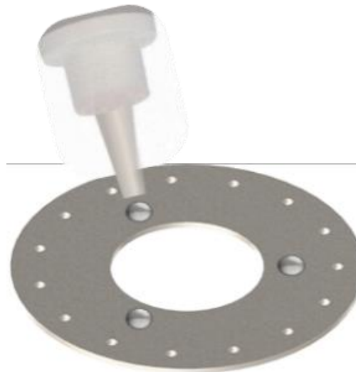
Figure 16. Where to add oil to the stainless-steel impaction substrate.
