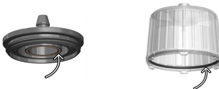
(a) GEN1 Flow Check Adapter 20-mm ID × 1-mm CS Viton™ (75A) (b) GEN2 Flow Check Adapter 43-mm ID × 1.5-mm CS Buna-N (70A)
