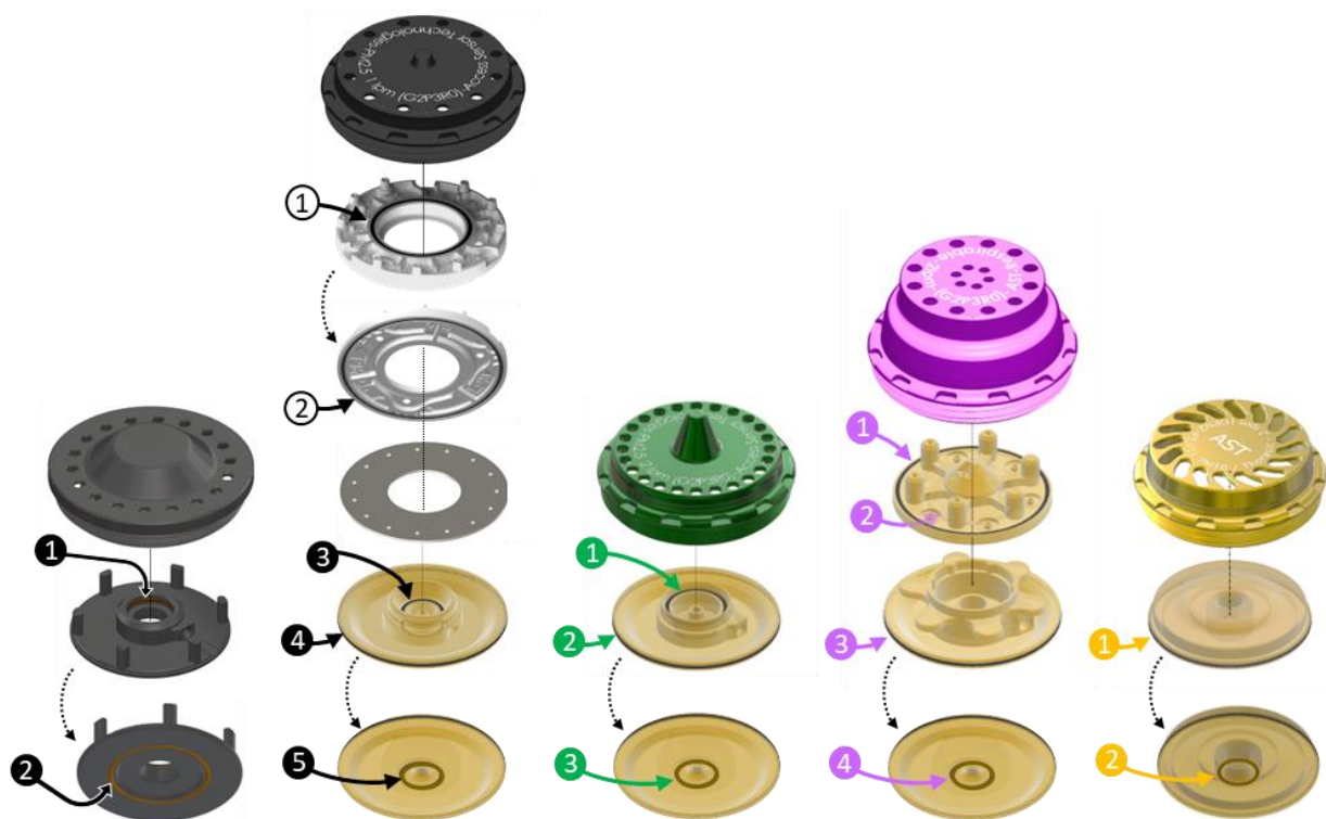
Figure 28. The location of each O-ring in each size-selective inlet.
